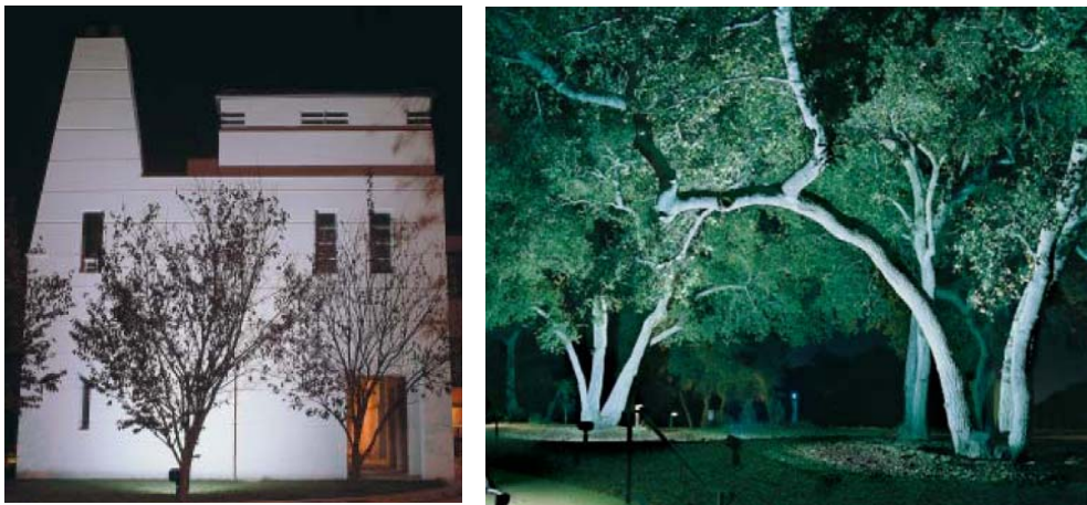
Figure 10- Installations using high wattage floodlights are only allowed in lighting zones 3 and 4. ( Left ) building façade lighting and ( right ) commercial landscape lighting (Kim Lighting)
