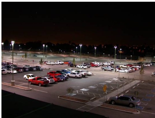
Figure 4 - Every Other Row Option Parking Lot with Fully Shielded Luminaires ( Monrad Engineering, Inc. )
