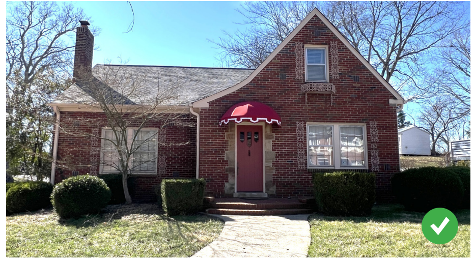
This Tudor Revival house is located at the corner of Anderson and McClure Streets. Even though the chimney is not integrated into the design of the front facade as with many houses of this style, its height still has prominence that is characteristic of the style.
