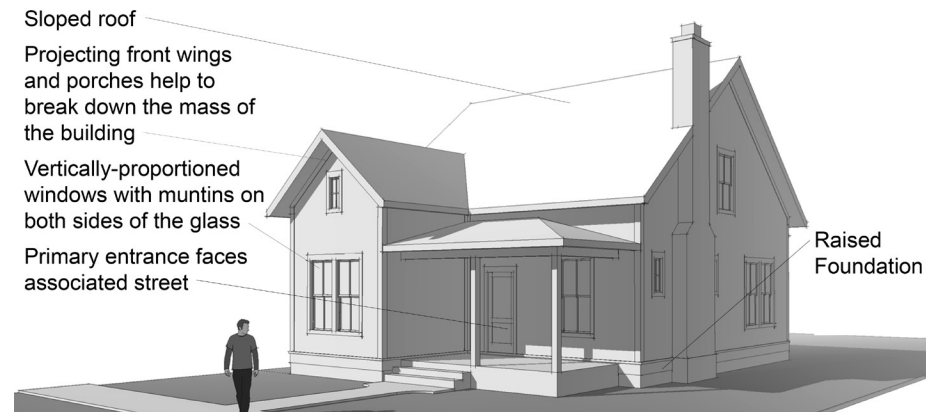
This diagram illustrates some of the common elements of new single-family detached residential buildings in historic neighborhoods.
